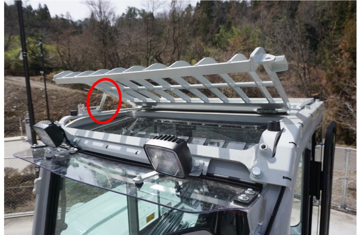
To close the guard, raise the guard and pull the stopper.
