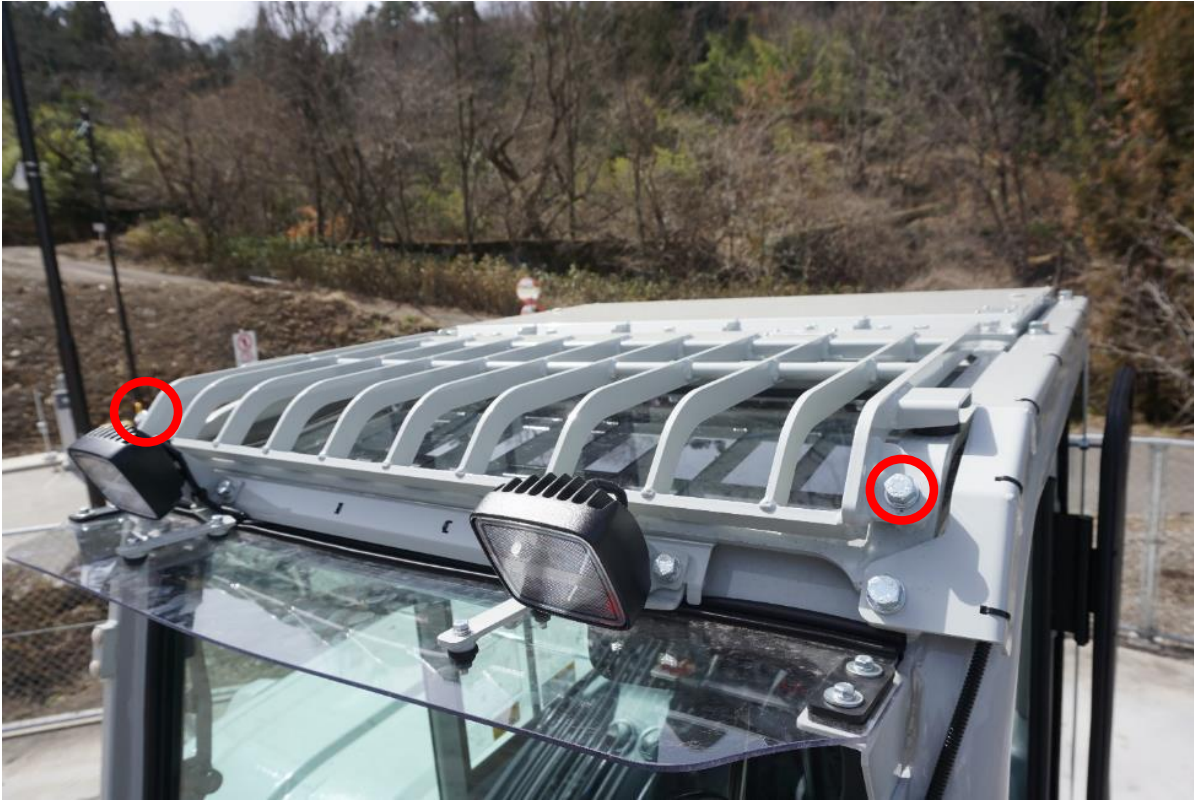
Remove two bolts to raise the roof guard.
